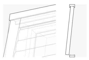
Push the bottom of the panel back into window until it slots into the bottom channel.
