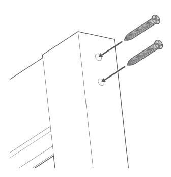
Secure the top bars using 2 screws per side.
