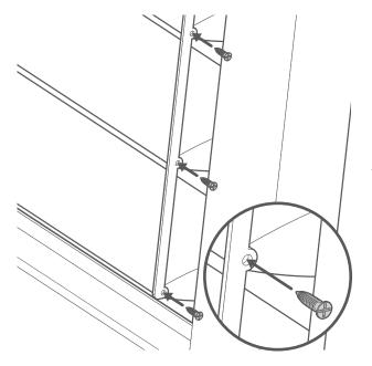
Take the hidden tilt bar and screw it into place on the back of the louvres, using the pre-drilled holes in the end of the louvres.
