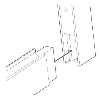
Slot the bottom bar into the side stiles. The end of the bar, and the inside of the slots in the stiles, are marked to help you locate them correctly.
