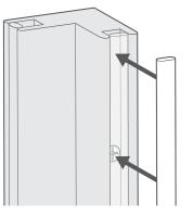
For Inside Recess frames, reinsert the decorative strips you removed in step 2.
