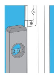
Make sure you also use the spirit level on the front of the frame, on all sides, to ensure there's no 'twist' to the frame.
