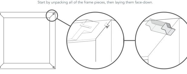
Line up all the corners, then insert the Hoffman keys from your fittings kit to join the frames securely together. The key can be a little tight, so you may have to give it a few taps with a hammer to fully insert it.
