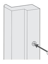
For Front of Recess frames, use the supplied screw covers to cover the screws.
