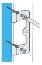
Start by loosening the frame hinges, as this will make aligning the two parts of the hinge easier (one part is fixed to the frame, the other part is fixed to the panel). This will also allow you enough room to slot the hinge pins into place.
