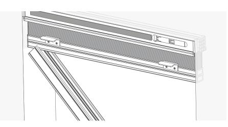
Holding the channel at an angle, align the open face of the channel over the blind's bottom bar.
