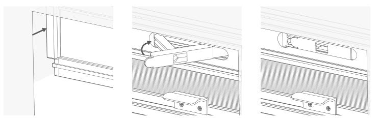
Leave a space of around 10mm between the front of the blind and the edge of the recess, so that there's space to fit the pelmet on the front later. Ensure that there is a gap of at least 50mm between the back of the blind and the window frame.
