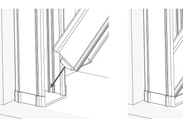
Insert the bottom bar into one of the side channels, with the bar angled up at the other end.
