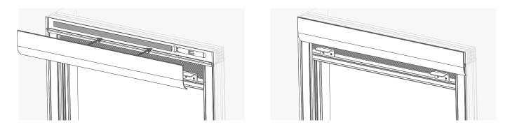
Finally, attach the pelmet to finish. The pelmet simply attaches with magnets, just line up the magnets on the back of the pelmet with the strip on the front of the blind's headrail and press into place.
