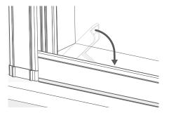
Push the raised end of the bottom bar firmly down until the bar is flat and level. Lock it into place by pushing the locking lever down until it snaps into place.
